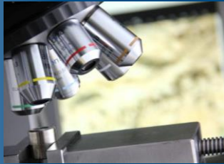
3D microscope InfnitFocus Alicona 25 to 1000x amplification
