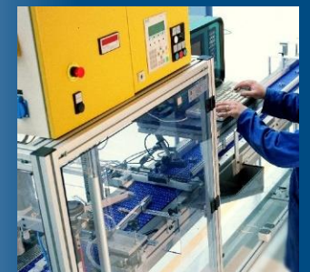
Automatic vibration/noise test (GP1)
